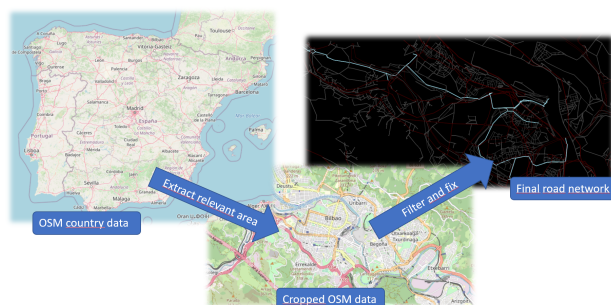
Figure 2: (1) The country wide map is retrieved from OSM. (2) The relevant area is extracted. (3) The map data is filtered and the minimal road network is stored.
